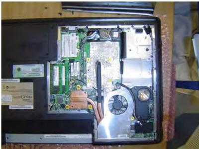
After having removed the heatsink, two more screws keep the MXM on the motherboard. Remove them and then take out the 6800. When you place the x1800 against the heatsink, you will notice that one of the coils (square blocks) on the MXM card interferes with the heatsink.
